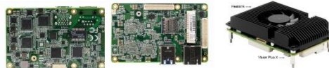
Customized card based on Intel® Movidius™ Myriad™ X VPU: AAEON UP AI Vision Plus X
